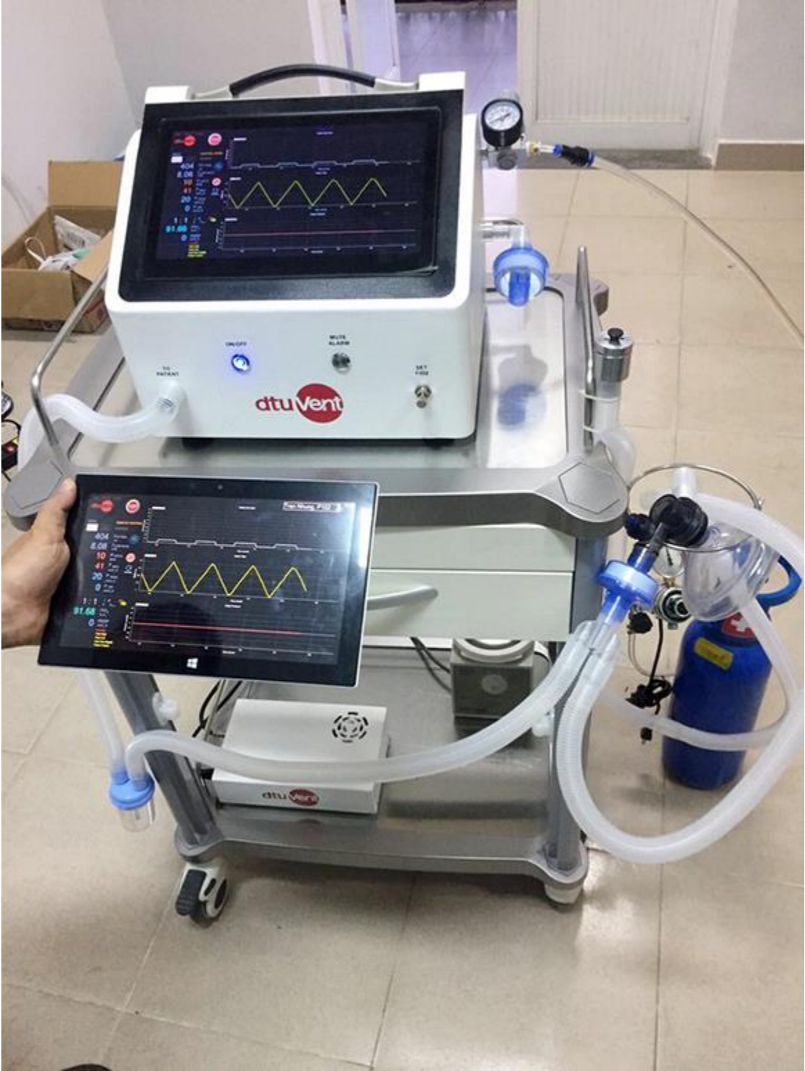
DTU-Vent version 2.0, the “2-in-1” ventilator
