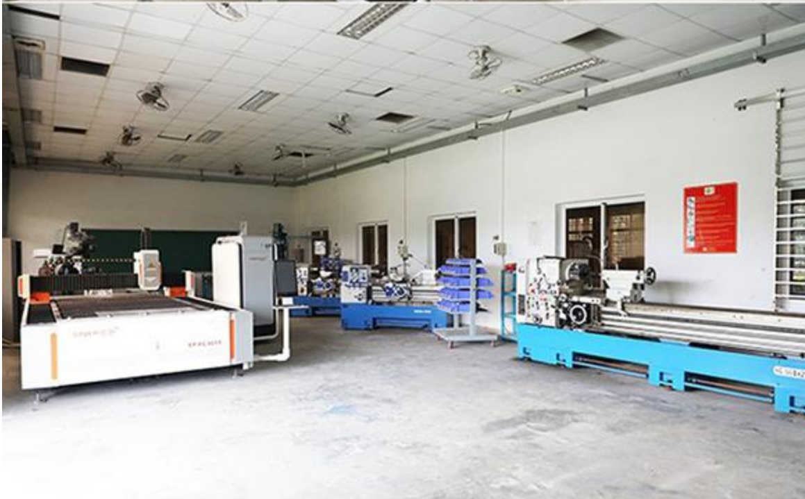
CNC machinery (above) and a mechanical workshop, with a lathe and a laser cutting machine
