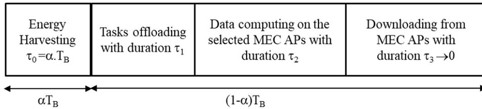
Figure 2. Time flow chart for proposed protocol
