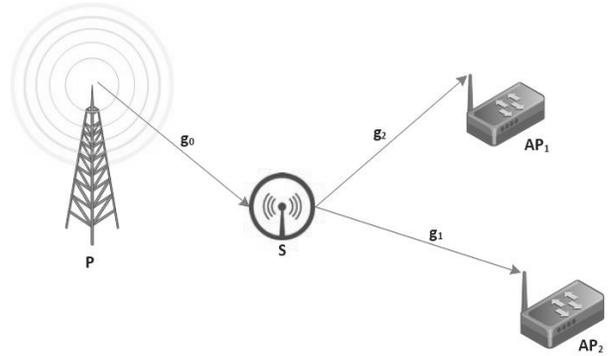
Figure 1. System model for RF EH NOMA MEC network
