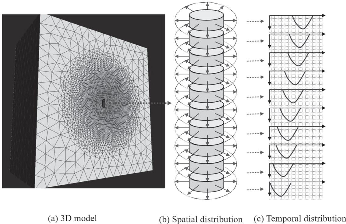
Figure 1: Three dimensional modelling and boundary condition setting
